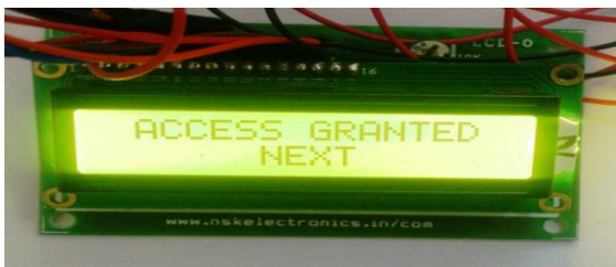
Figure 3: LCD displaying “ACCESS GRANTED” after the unique ID number entered by user is confirmed as valid number, and “NEXT” is being displayed for allowing next person to enter his/her unique ID number.
