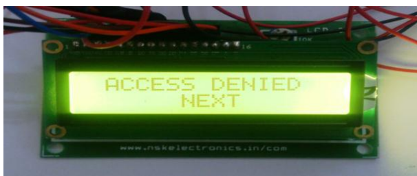
Figure 4: LCD displaying “ACCESS DENIED” after the unique ID number entered by user is confirmed as not a valid number, and “NEXT” is being displayed for allowing next person to enter his/her unique ID number.
